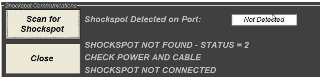
If you get this message when you click the connect button the most likely problem is that the driver is not installed for the Shockspot communication hardware. The drivers for Windows 7 through 10 are included in the Shockspot setup files.
